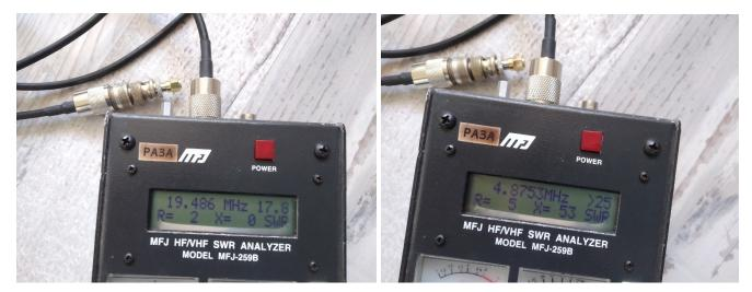
For measuring at 1/8 wavelength, the frequency must be 4x lower than that for  $\frac{1}{2}$  wavelength, so approx. 4.875 kHz. The reading on the MFJ is now: Z = 5 + j53. The characteristic impedance of the cable is then | Z | = square root (25 + 2809) = 53.2 ohms. According to the specs, a Belden RG-58/U would have a characteristic impedance of 53.9 - j2 ohms. Right on target. *The MFJ-259B did it again!*
