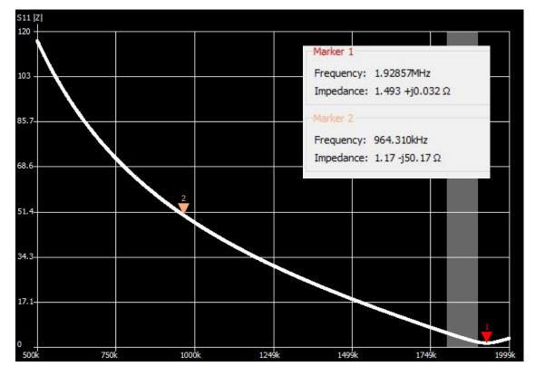
The red marker with no. 1 is at the frequency where the impedance is low/almost zero and practically ohmic (so not inductive or capacitive): 1928 kHz. At this frequency the electrical length of the cable is therefore 1/4 wavelength. So we don't need to know the exact length of the coax, nor the exact velocity factor, it is just ¼ wavelength long for that frequency. If you cut the frequency in
