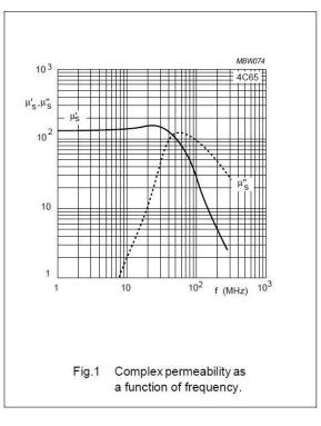
We can extract three important measurement points from this to identify a core:
