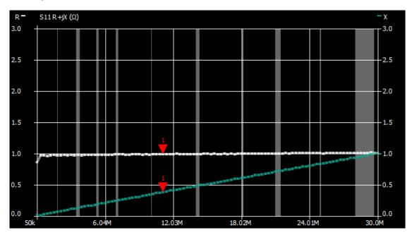
We can see that the value of 1-ohm is displayed correctly over the entire HF range (between 0.97 and 1.01 ohm) and that there is a linearly increasing reactance. In nanoSAVER you can read that it is about 5nH, reasonable for just average simple resistance. We can therefore cautiously conclude that with a few percent measurement tolerance you can still measure sufficiently well up to 1-ohm.
